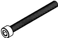
Fig. B M6 Socket head cap screw, QTY: 4
